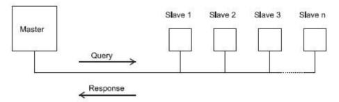
In the MODBUS Protocol the master can address individual slaves, or, using a special "Broadcast" address, can initiate a broadcast message to all slaves. The Reltech Digital meter do not support the broadcast address.
